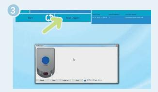
After the test program is completed, place the SteriSense measuring device back in the reader station to **read the data**.
