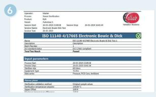
The test results will be stored in the software and be included in an automatically generated PDF report.
