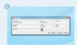
Place the SteriSense measuring device in the reader station and open the SteriSense Software. Define a unique Session Name.
