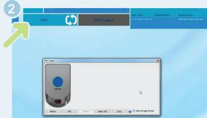
Press **Start** to activate the SteriSense measuring device, and place the device inside the steam sterilizer.
