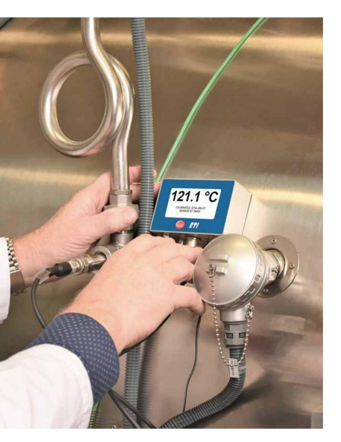
FDA compliant alternative to mercury-inglass thermometers for retort monitoring - and much more
