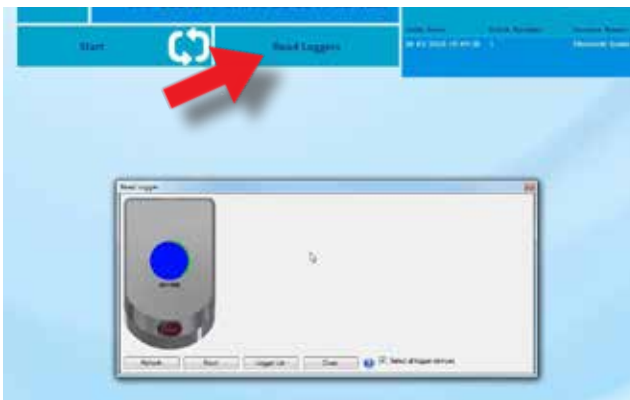
After the test program is completed, place the SteriSense measuring device back in the reader station to read the data.
