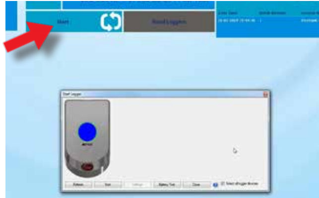
Press Start to activate the SteriSense measuring device, and place the device inside the steam sterilizer.
